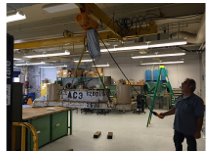
Successful crane load testing
